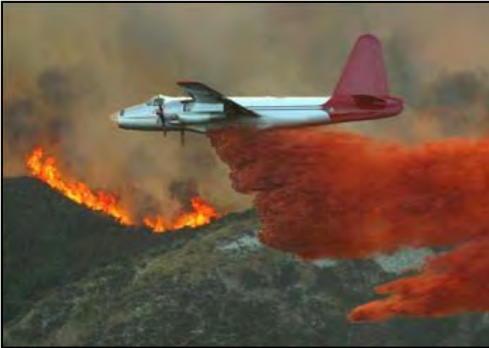
The P-2V Neptune is an old U.S. Navy antisubmarine warfare aircraft used for wildfire fighting. U.S. Forest Service photograph
