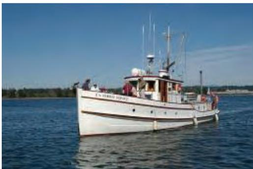
carvel-planked "survey" vessel with a raked stem, round bilge, a full keel, and a round stern. It is arranged with a raised foredeck that carries a raised pilothouse. The side decks are dropped 21 inches at the back of the deckhouse where the main cabin carries toward the stern and the aft deck. One galley, one head, and eight berths are found inside.
