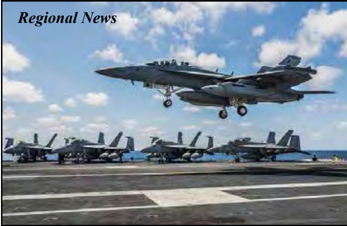
The EA-18 Growler has replaced the EA-6B Prowler as the U.S. Navy's carrier-based electronic warfare aircraft.
